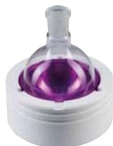
Reaction block, 500 ml H 135.5
